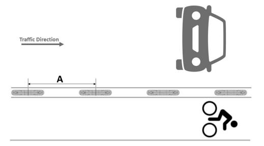
The parallel positioning of TreeTop Premium Rubber Bike Lane Delineators is most suitable when there's limited available buffer zones (i.e.; painted lines). To ensure optimal safety, it is recommended to maintain a spacing between centers (A) of 6ft between the delineators, while not exceeding 8ft.
