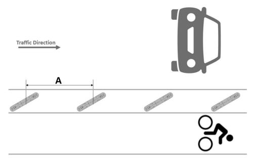
The oblique positioning is recommended when you need to create a wider buffer space for enhanced safety in the bike lane. A wider buffer zones (i.e.; painted lines) contributes to greater safety for cyclists. To ensure optimal safety, it is recommended to maintain a spacing between centers (A) of 6ft between the delineators, while not exceeding 8ft.
