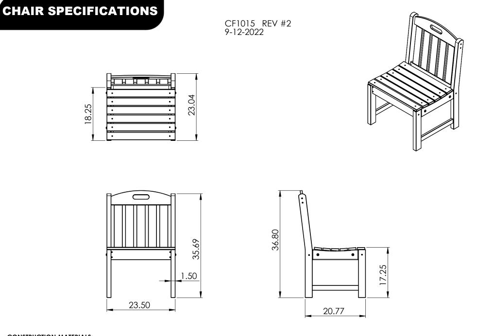
CONSTRUCTION MATERIALS: Recycled Plastic HARDWARE: Stainless Steel
