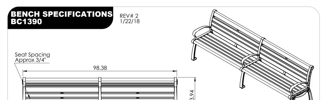
Back Spacing Approx 7/8" Tear drop board 3.75" x 1.34" 2.88" of flat surface on board Bull nosed board 3.75" x 1.34" 3.00" of flat surface on board Square board 2.36" x 1.34"  $^{\circ}$
