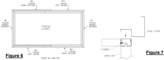
Place a double mitered fascia #1 on a short side of the shelter. The mitered ends of this piece will be visible when looking up at the bottom of the fascia. Repeat process on the other short side of the shelter. **See Figure 7**.
