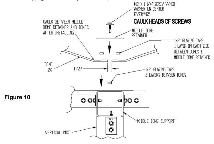
Install the perimeter dome retainer (1" x 2 1/2" x 1/8" alum angle) around the perimeter of the shelter using #12 x 1-1/4" hex head with neoprene washer self tapping screws, 12" on center. **See Figure 10.**
