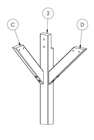
Note: Do NOT attach boards C or D where there are no pilot holes. Follow the pilot holes
