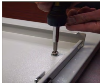
Figure 8: Attaching the sign bracket.
