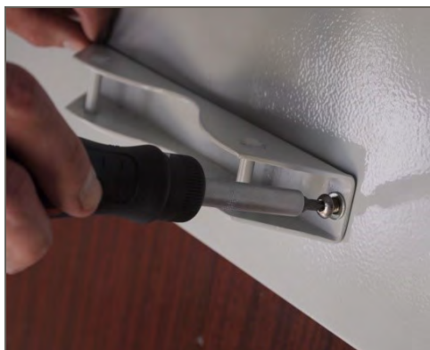
Figure 5: Attaching the banding bracket to the sign
