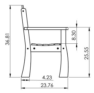
CONSTRUCTION MATERIALS: Recycled Plastic HARDWARE: Stainless Steel
