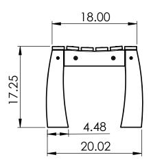
CONSTRUCTION MATERIALS: Recycled Plastic HARDWARE: Stainless Steel
