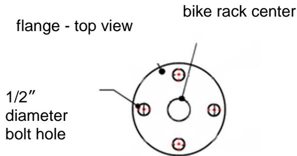
**Note:** Surface mounting hardware sold separately. Use 3/8" x 4" lag bolts. It is recommended that concrete cure 28 days prior to mounting.
