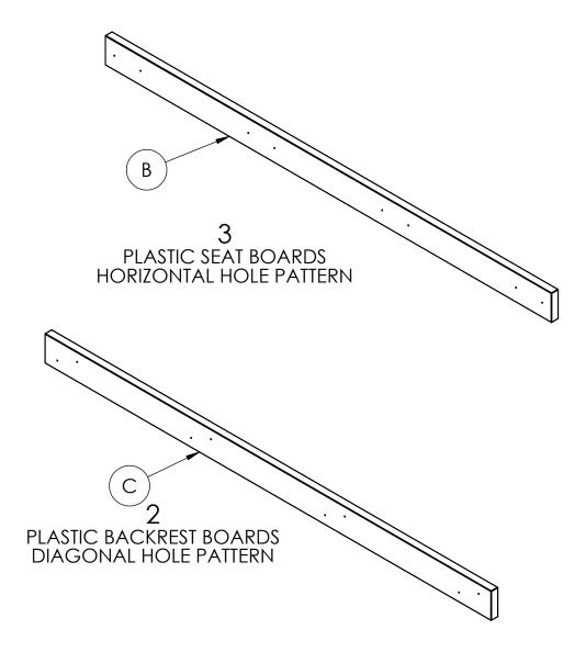
NOTE: IT IS IMPORTANT TO KEEP ALL SCREWS LOOSE DURING ASSEMBLY UNTIL ENTIRE BENCH IS ASSEMBLED
